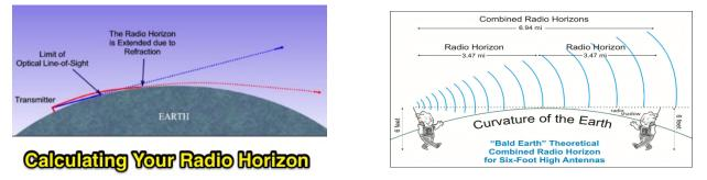
The *radio horizon* is the locus of points at which direct rays from an antenna are tangential to the surface of the Earth. If the Earth were a perfect sphere without an atmosphere, the radio horizon would be a circle.
